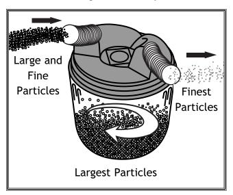
Figure 22. Dust Collection Separator.
